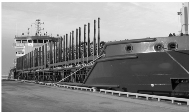
Figure 6.9. Uprights for blocking over the entire height of the stow
